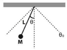
The pendulum consists of a massless, rigid bar with a length L, and with a mass m hanging at the end. We assume that there is no friction acting on the motion of the pendulum (no damping).
